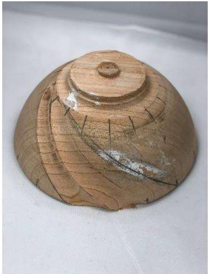
Once the blank has been marked with index lines, AI selects an off-set value to set the pitch for the “helical curve”. The curve is laid onto the bowl surface using a gauze plaster bandage that marks the curve. The bandage dries quickly and is transferred between index points to enable creation of uniform layout lines. Much faster than hand plotting each curve!
