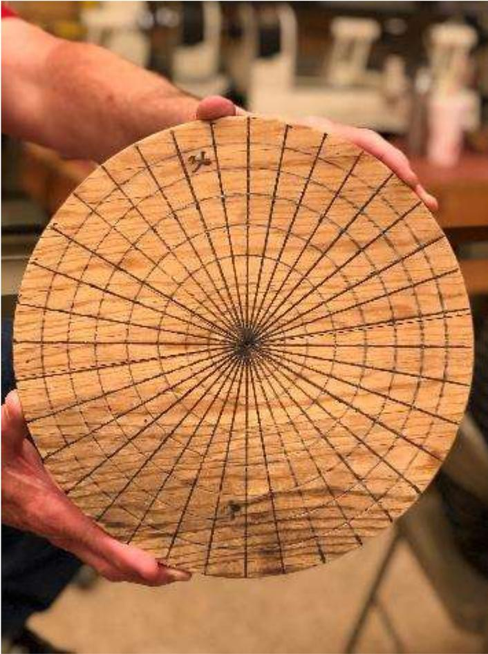
Index plates are used to lay out the flute spacing and texture blocks after the bowl is roughed out. The bowl can be laid on the plate and quickly divided. Shown here is a 36 segment plate. The radial lines are bisected with rings that can be used to center the object on the plate and index spacing as desired.
