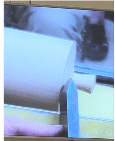
Using the tool point to sharpen the corner and add a bead
